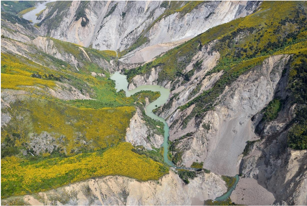
Figure 4: Landslide dams in the upper reaches of the Conway River in the Seaward Kaikōura Ranges. Two landslide dams are visible in the photo with water still impounding behind both. The source material for the landslides is Torlesse Greywacke which typically forms disrupted rock slides because of the closely jointed and fractured nature of the source rock mass. The resulting debris can be described as an angular gravel and is highly permeable. As a result, none of the large greywacke derived landslides overtopped under non-flood conditions, but developed flows through the permeable material forming the dam. (Photo: D. Townsend, 16/11/2016).
