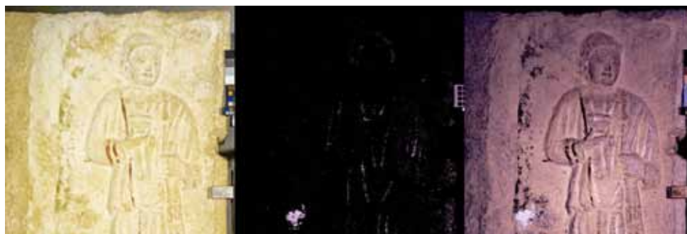
Figure 1. Visible (left), infrared luminescence (middle) and CoRL (right) image of a side element of a Roman funerary aedicula displayed in Mauerbach Charterhouse, depicting a male servant. White areas in the latter two images indicate the presence of Egyptian blue pigment.
