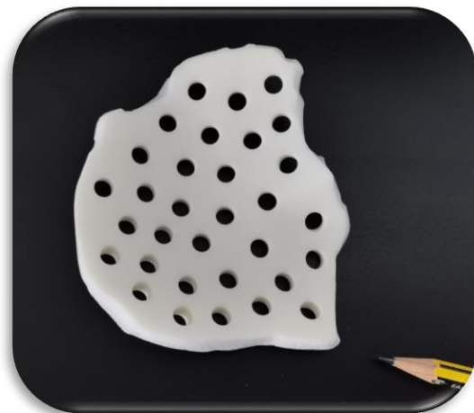
Figure 1: Sintered 3D printed skull implant
