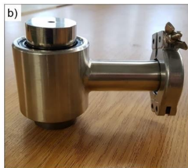
Figure 1. (a) Sketch and (b) photograph of sealed chamber to allow powder to be transported in local argon atmosphere to the HPT device.
