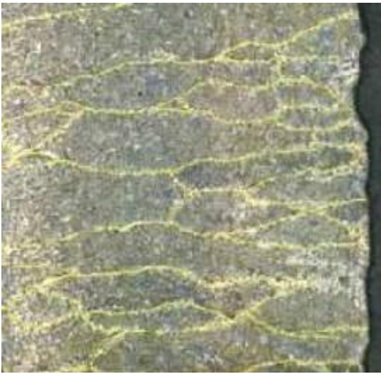
Fig. 3: A sample of a slab edge area. The austenite grain boundaries are highlighted by a yellow line.
