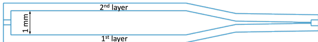
Fig. 13: Two-layered custom shape for cutting out optimized APT blanks with a fs-laser.
