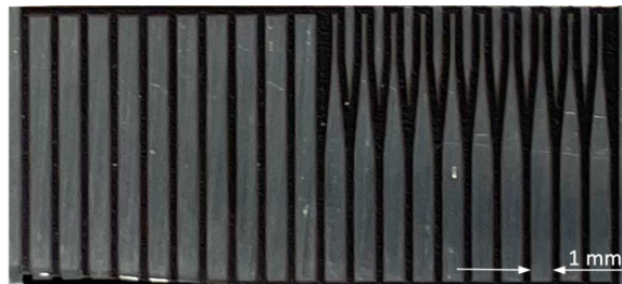
Fig. 20: Image of the result after cutting 20 APT blanks with a fs-laser ablation system out of a 1 mm thick Fe sheet, after cleaning with CO 2 snowjet.
