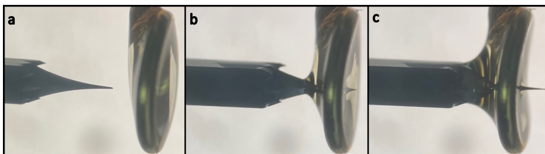
Fig. 31: Photographs through the LOM in the etching lab during step 2 micropolishing of a top-down circle ablation specimen with 60 \mu\text{m} inner pattern diameter without removal of secondary apexes, with (a) directly before step 2, (b) and (c) during step 2 after 2 min of preparation time, demonstrating capillary forces between the electrolyte and the secondary apexes.
