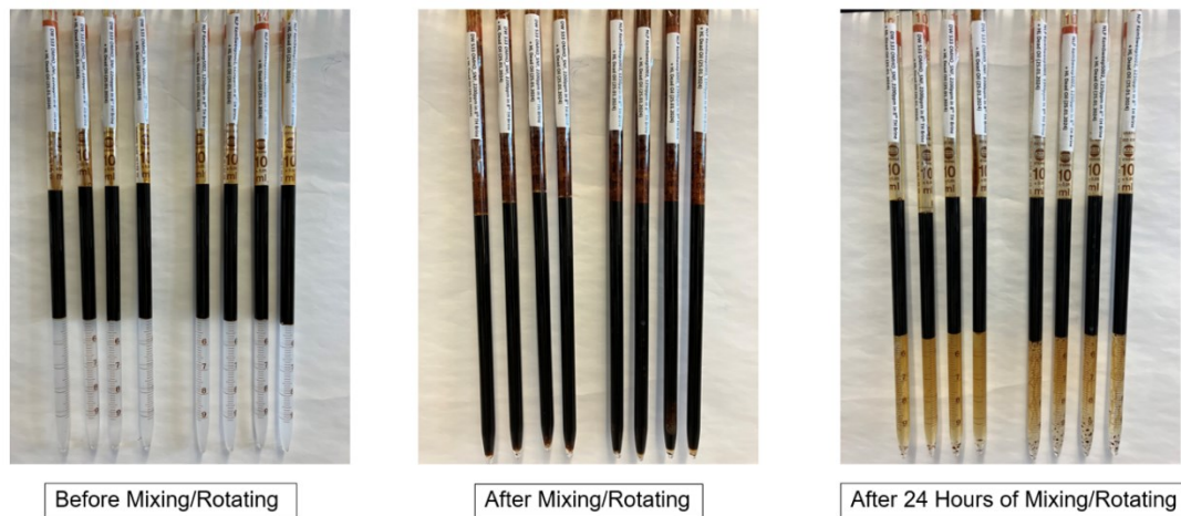
Figure 3.10 - Phase behavior test using pipettes to produce the emulsions resulting from fluid-fluid interaction. The left side of the four pipettes is for LP#1, and the right side of the four pipettes is for LP#2
