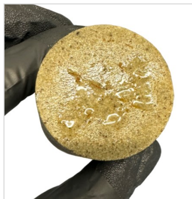
Figure 3.13- Filtration issue in 300mD core
