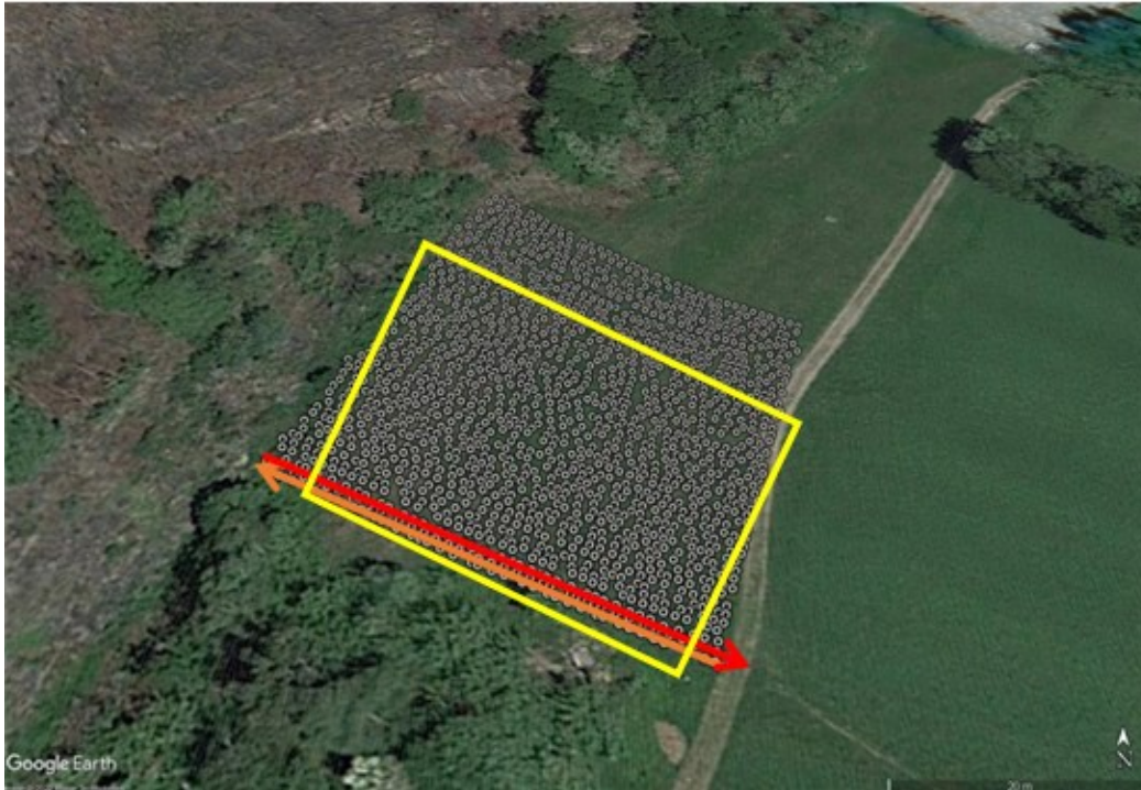
Figure 7.2: This figure is a map view of the GPR survey area to show where it overlaps with the Seismic Survey of the DT-1B drill site. The yellow rectangle approximately displays the Seismic Survey. The white and black circles represent the GPS locations of the data points gathered from the 250 MHz measurements. The orange arrow indicates what is saved in the data recording as the Uphill direction, and the red arrow indicates what is saved in the data recording as the Downhill direction modified from (Greenwood., 2023).
