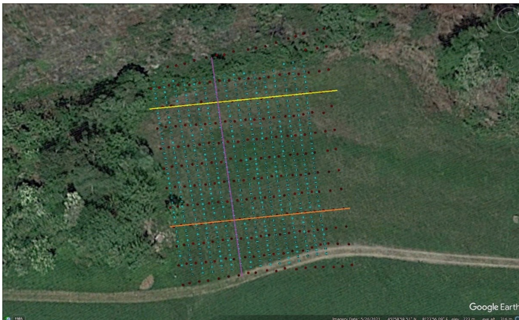
Figure 6.1: Map view of the survey site [Image @ 2023 Maxar Technologies]. Blue circles are the GPS coordinates of the receiving geophones. Red circles are the GPS coordinates of the shot locations. The yellow line represents the profile of Hard Rock Cross Line 35 in the survey. The orange line represents the profile of Soft Rock Cross Line 11 in the survey. The pink line represents the profile
