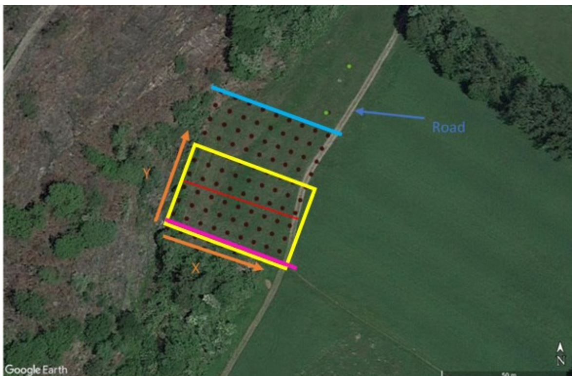
Figure 7.1: This figure is a map view of the ERT grid which overlaps the Seismic Survey of the DT-1B drill site. The yellow rectangle approximately displays the Seismic Survey. The dark red dots mark the GPS electrode locations, and the green circles are the GPS remote electrode locations. The Orange arrows present X and Y axis of the grid. ERT Profile Line 1 is represented by the pink line, and ERT Profile Line 20 is represented by the light blue line. The red line indicates the position of the aforementioned 237-meter length 2D profile where it overlaps the seismic and ERT surveys. The blue arrow indicates the footpath that is referred to throughout the survey modified from (Greenwood., 2023)
