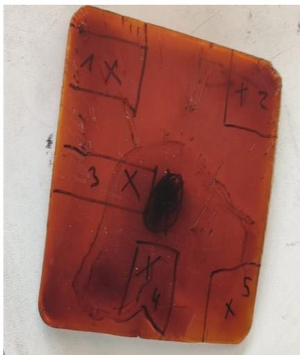
**S16.2** Image of a Limestone-RCFP resin cured in a PTFE mold. The portions on the cured plate from where samples were taken for DSC and FT-IR ATR measurements are labelled.
