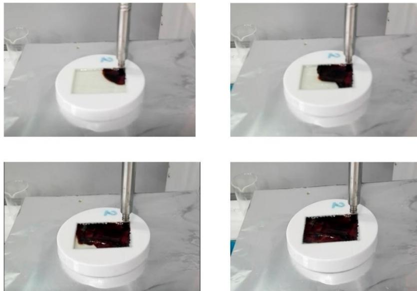
**Fig. 13** RICFP of a glass fiber reinforced composite initiated with UV light (picture courtesy of Sangermano et al. [57]).
