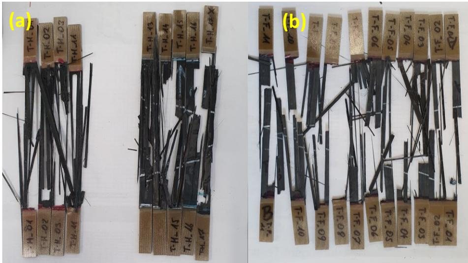
S7.4 (a) Images of tested tensile specimens cured via NR route and (b) specimens cured from NF route.
