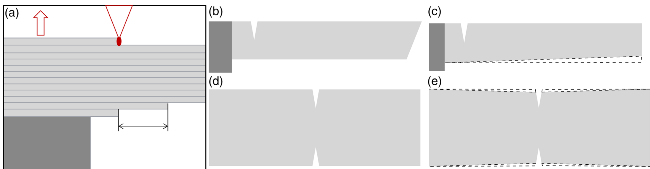
Figure 2. a) Printing strategy to overcome printing artifacts for large overhanging distances, with tapered geometry on faces pointing downward. Dark and light gray area indicates printed structure and layers. In red, printing from bottom to top with voxel and beam path for two-photon polymerization is indicated. Thereby, the overhanging distance at initially printed layers is reduced, decreasing the tendency of floating out of place before subsequent layers are cured. b) Side view of ideal notched cantilever and under c) a version prepared with the printing strategy depicted in (a), with changes (dashed line) aiming for a precisely defined physical specimen. For the double notched tension geometry in d), the same approach is applied in e) on the upper and lower side to preserve the symmetry.
