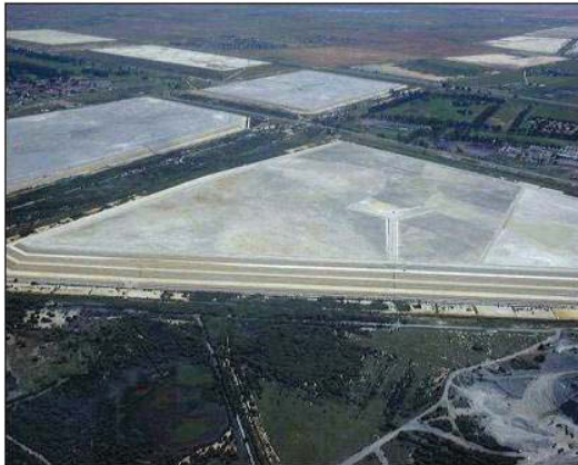
Fig 13: Picture of a tailings pond built on flat land [9, European Commission, 2009, p.73]
