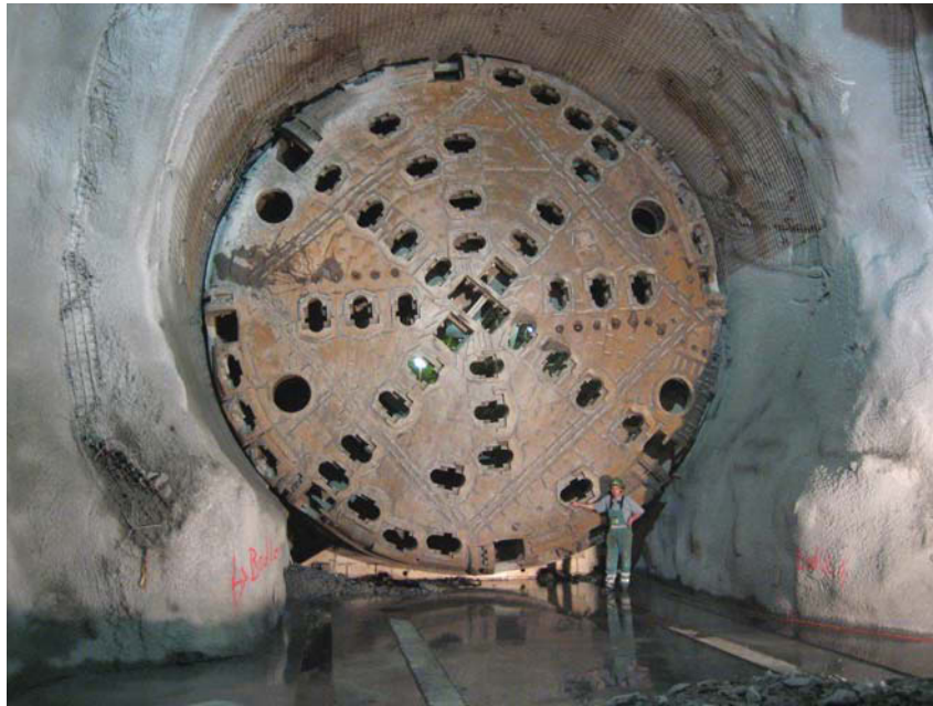
Fig. 3.1: Front of a Tunnel Boring Machine (TBM), [27].
