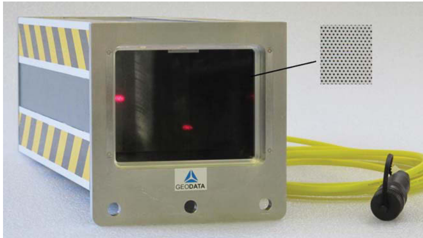
Fig. 1.1: A prototype Active Laser Target. This device was designed for the guidance of tunneling machines. Upper-right: Enlarged dot-pattern on semi-transparent target. (Photograph by Geodata GmbH [11]).
