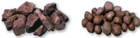
Figure 5: Lump ore and pellets used in MIDREX process [8]
