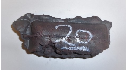
Figure 74: Briquette showing typical signs of segment wear
