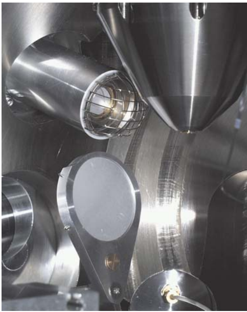
Figure 5-2 The lower part of the objective lens (up), SE detector with collection grid and the phosphor screen.
