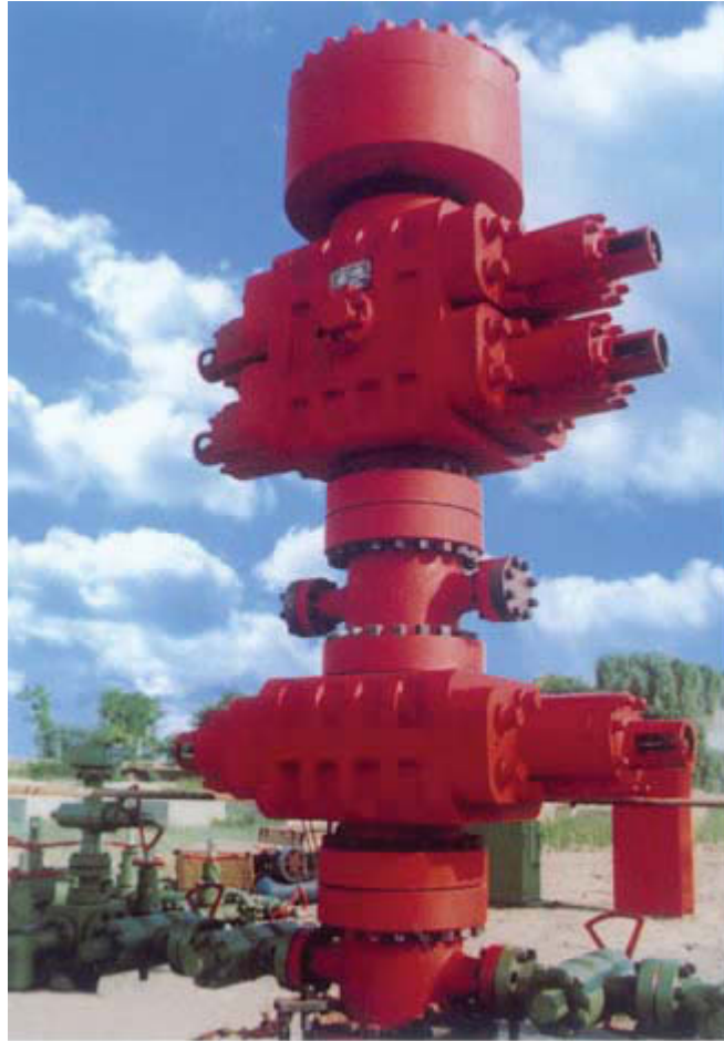
Figure 2 Surface mounted BOP stack [2]
