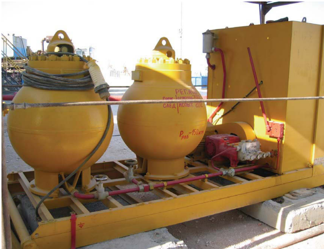
Figure 13 Accumulator unit with spherical bottles (not in accordance with API)
