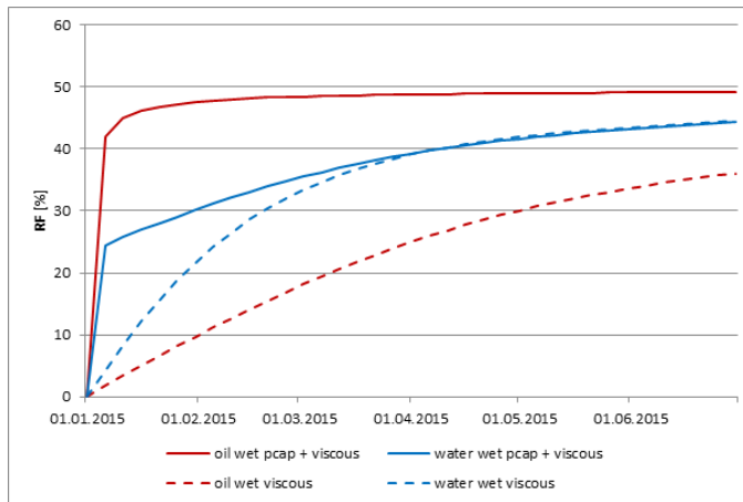
Figure 4.3: Results for Water Injection Only. Significant differences can be seen between the individual curves. Wettability as well as driving mechanisms have influence on both shape and ultimate recovery after six months.
