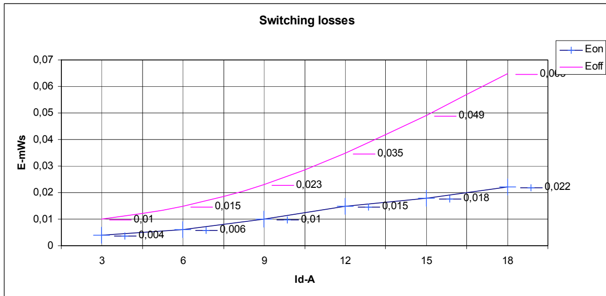
Figure 4-26: Switching losses in power devices ( E_{on}+E_{off} ). E_{on} includes SPP20N60C3 diode commutation losses. E = f(I_d) , inductive load, T_j=125^\circ\text{C} , V_{ds}=380\text{V} , V_{gs}=0/+13\text{V} , R_g=3.6\ \Omega
