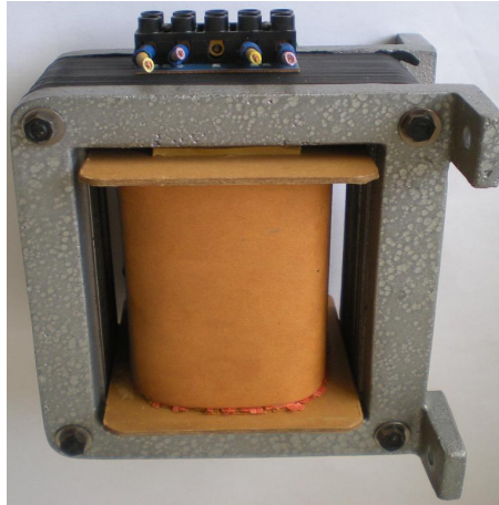
Figure 5-24: Single-phase, 220V, 200VA, 50-Hz transformer
