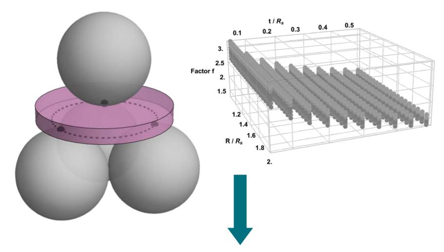
$$f_{B3B} = Exp \left[ c_1 (1+v) + c_2 ln \frac{t}{R_s} + c_3 \sqrt[4]{\frac{Rt^2}{R_s^3}} \right]$$
