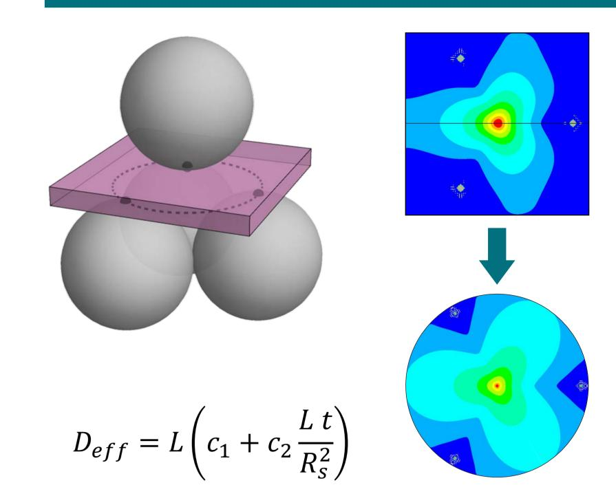
The edge length L is converted to a diameter  $D_{\it eff}$  of an "effective disc" to allow stress evaluation with the new fit for  $f_{\it B3B}$ .
