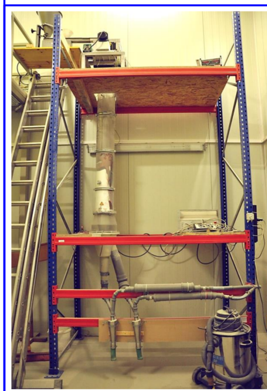
A prototype of the coaxial triboelectrostatic separator [4]
