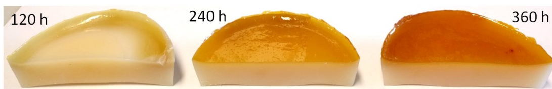
Figure 5.5: Cross sections of the HDPE specimens after 120 h, 240 h and 360 h of static thermal exposure at 160 °C in air. The extent of discoloration increased with increasing exposure time. Dark spots on the surface were attributed to accelerated aging caused by catalyst residues.
