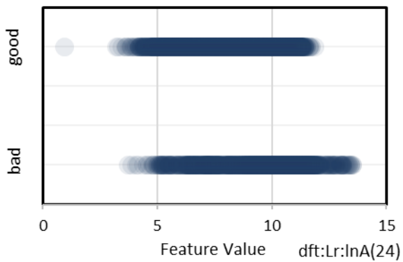
Figure 156: Descriptor (24), raw sucker rod load, natural log of amplitude spectrum
