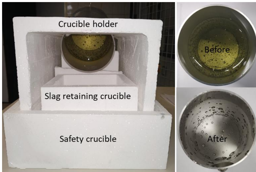
Figure 18: Setup for slag drain out at elevated temperature; crucible before and after drain out.
