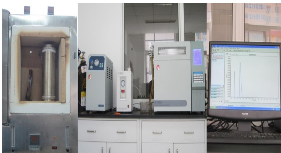
(a) Programmed temperature oven (b) GC-4008B gas chromatograph (c) Gas chromatograph analysis software
