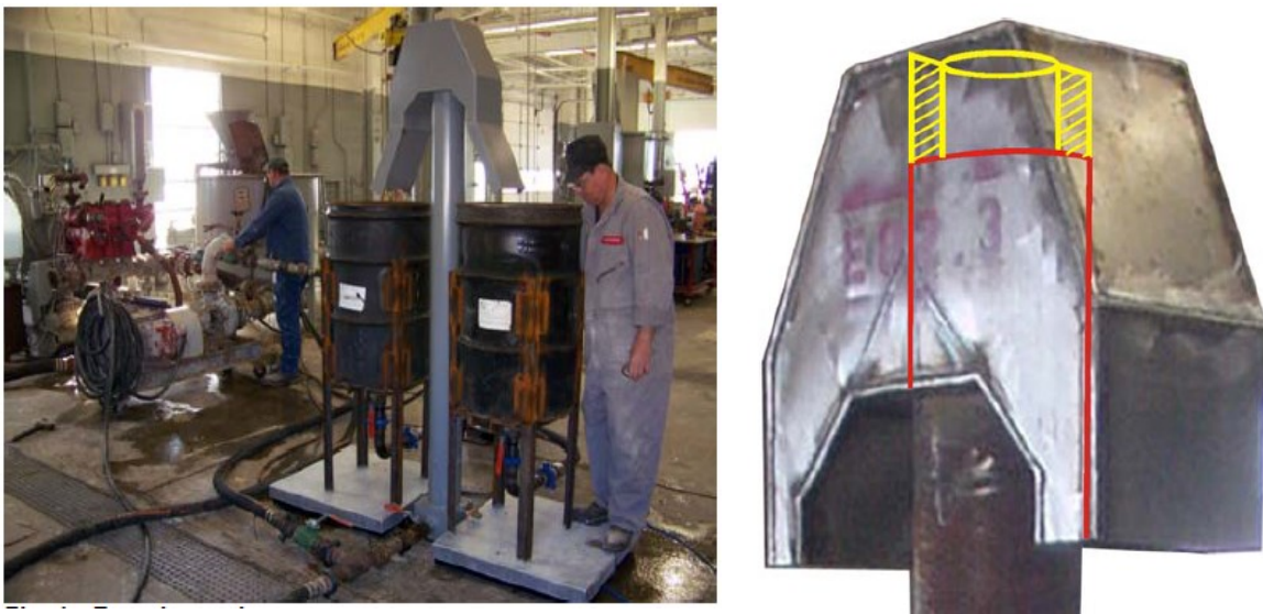
Figure 36. Experimental setup and measurement method for wide and narrow side velocities
