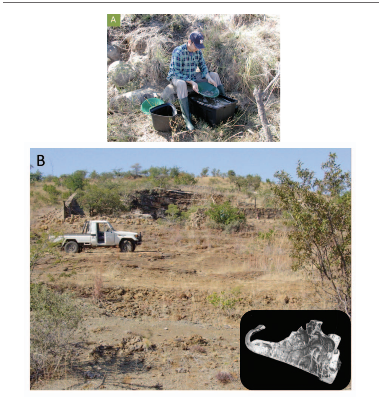
Figure 2. Field activities: (A) Panning of alluvial PGM, Dwars River, Der Broeben, south of dam. (B) Onverwacht Pipe (in the background), and eastern slope (foreground) that was sampled for eluvial PGM. Inset: largest (1.87 mm) eluvial PGM grain (Pt-Fe alloy) found at Onverwacht (grain 4/55).
