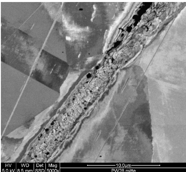
Fig. 5. SEM image (backscatter electrons) from part of the crack of Fig. 3.
