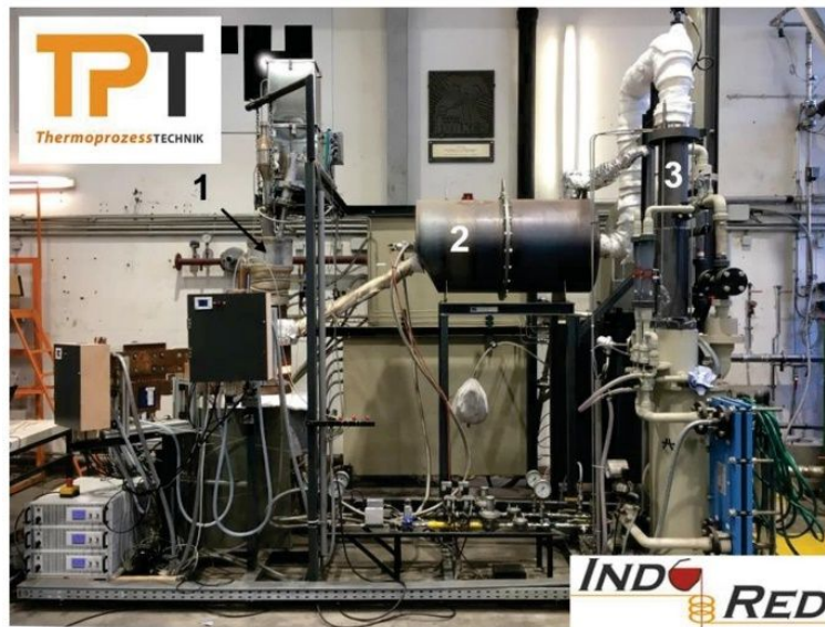
Figure 9: Main components of the InduRed pilot plant – (1) reactor, (2) post combustion chamber, and (3) gas scrubber [14]
