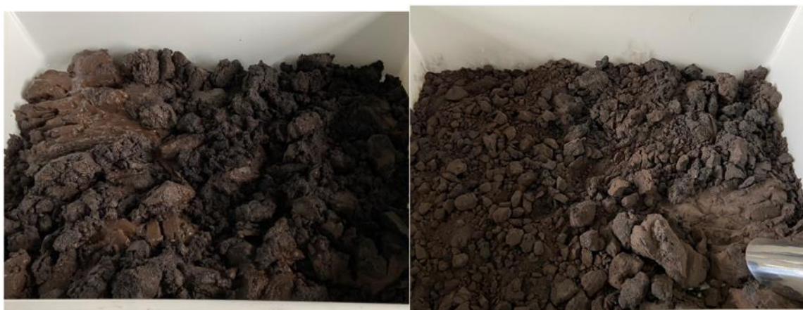
Figure 7. (a) Feed material at its initial condition and (b) Feed material after drying at 105°C
