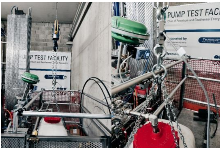
Figure 25: Flow Rate Measurement Setup (left) and Load Cell with Tank (right)
