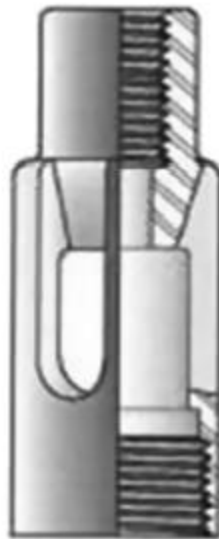
Figure 12: Standing Valve Open API Cage [1, pp. 80]
