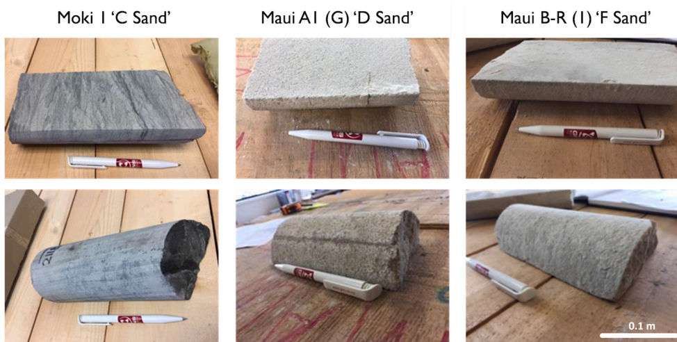
Fig. 3. Photographs of selected reservoir intervals from petroleum boreholes Moki-1, Maui-A1(G), and MBR (2) used to subsample core plugs for non-destructive and destructive laboratory testing.
