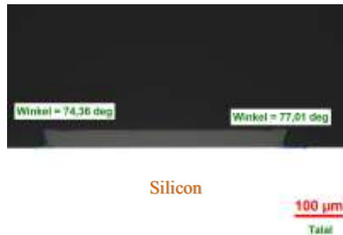
Fig. 9 Exposure energy: 45 mJ/cm 2 , Development time: 5:00 minutes
