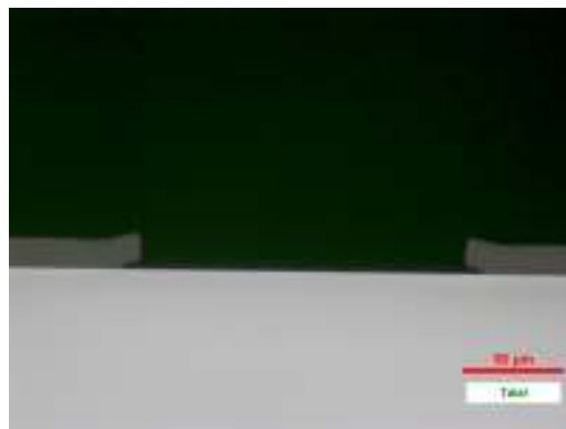
Fig. 13 Consistent resist lifting from silicon wafer
