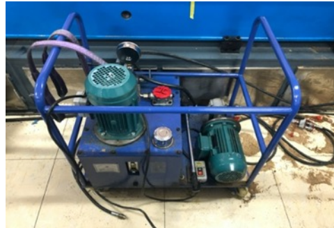
(c) Automatic closed-loop electro-hydraulic servo loading system
