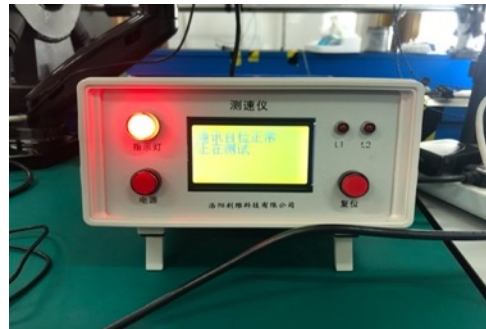
(b) SHPB special non-contact optical velocimeter
