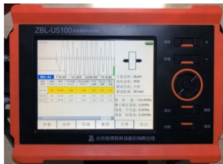
(a) Non-metallic ultrasonic velocimetry
