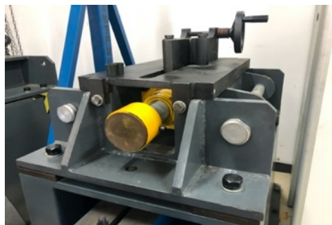
Fig. 2.8 The energy absorption device
