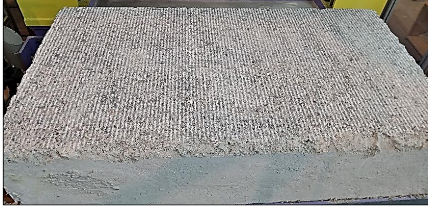
Figure 26. Conditioned concrete surface.
