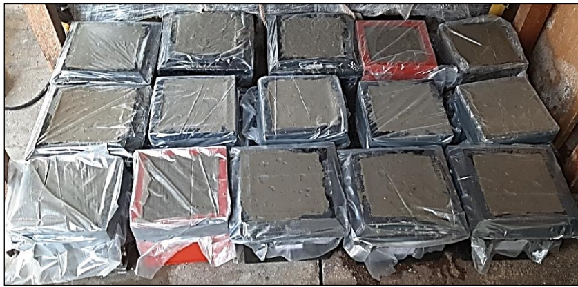
Figure 25. Cubic samples for UCS determination of concrete.
