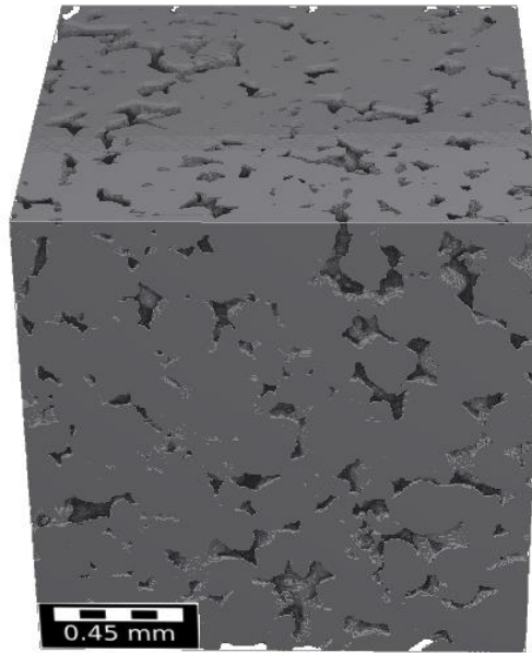
Figure 38. Berea_2 structure, used for deeper insight and relation of this and other studies using Berea.
