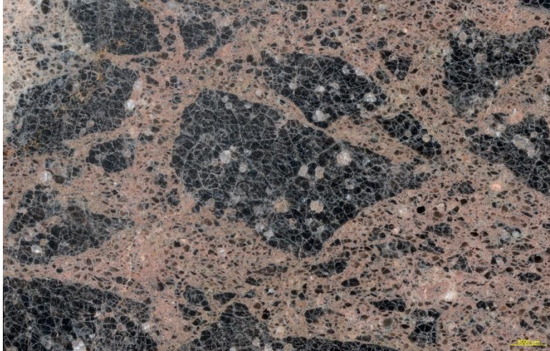
Fig. 19: Thin section of phreatic lava breccia with high degree of perlitic fractures; sample Ad-18.
