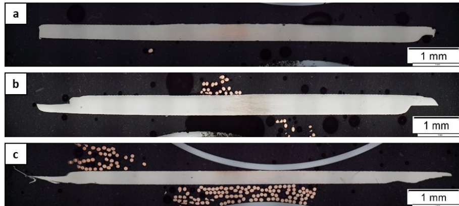
Figure A.1: LM images of the HPT sample cross-section of (a) \text{Cu}_{82}\text{Fe}_{12}\text{Co}_6 , (b) \text{Cu}_{60}\text{Fe}_{20}\text{Ni}_{20} , and (c) \text{Cu}_{80}\text{Fe}_{10}\text{Ni}_{10} after deformation for 100 turns at RT.
