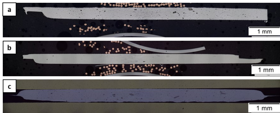
Figure A.5: LM images of \text{Ag}_{84}\text{Fe}_{12}\text{Co}_4 after deformation for (a) 100 turns at RT (untreated), (b) 100 turns at 300°C (untreated), and (c) 100 turns at RT (BMVA-pretreated).
