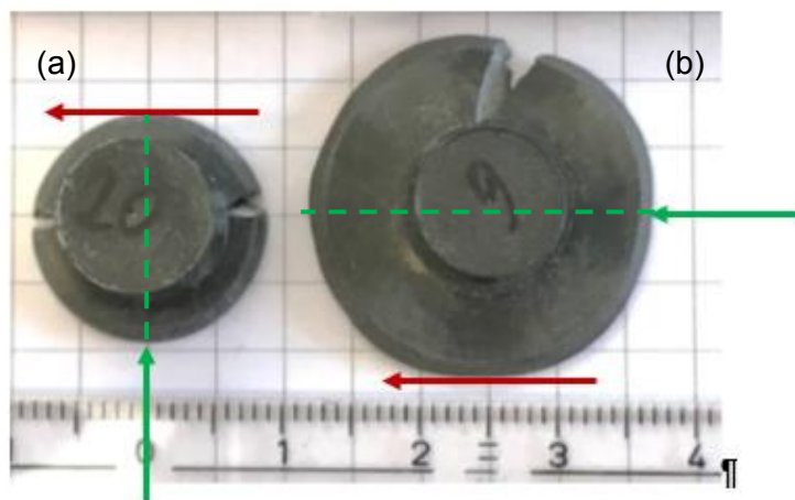
Figure 57: Cutting directions for cross section ion cutting – tangential (red arrows) and parallel (green arrows), (a) 27MnSiVS6, as-rolled, (b) 42CrMo4, annealed
