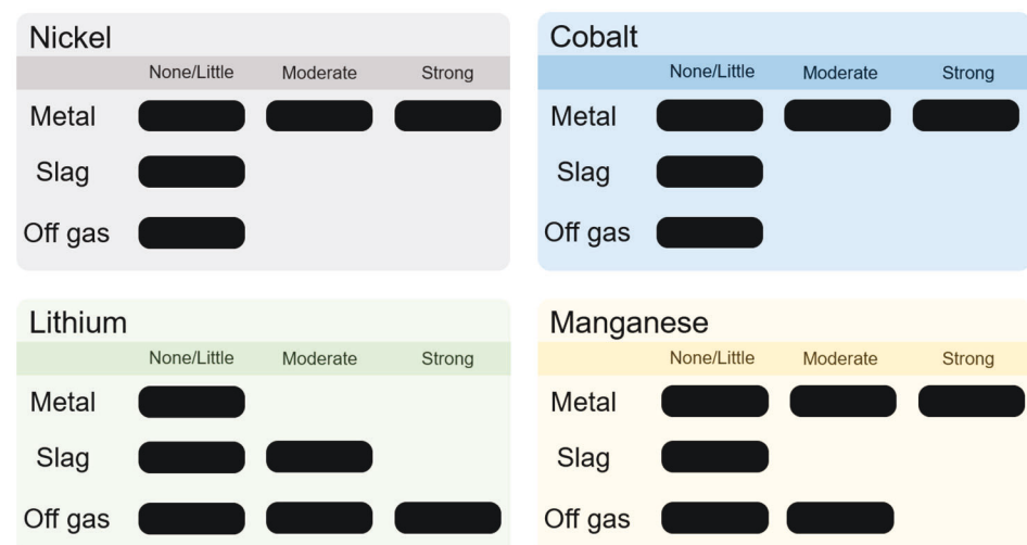
Figure 11. Qualitative consideration of the accumulation of Ni, Co, Mn and Li in the product phases obtained from the InduMelt experiments.
