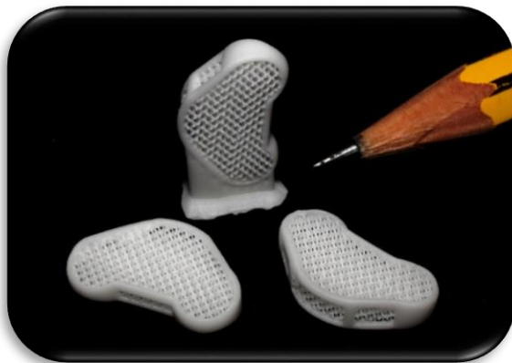
Figure 2: Spine implant with cellular structure
