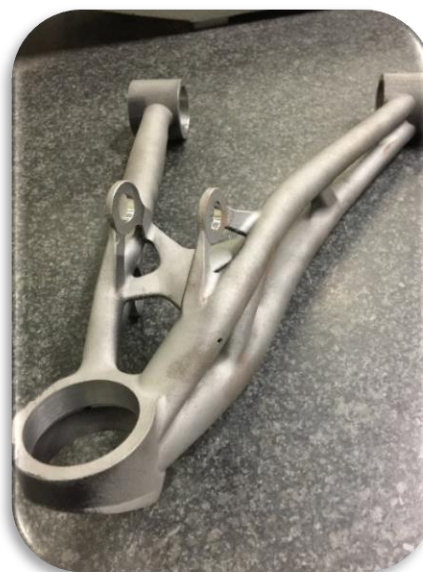
Figure 1: Demonstrator of the suspension arm showing the potential of AM production for automotive application
