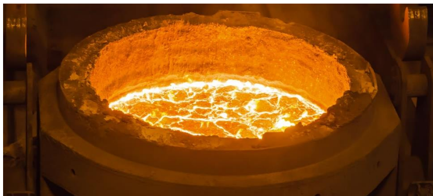
Figure 1: Refractories application (steel ladle) [4]
