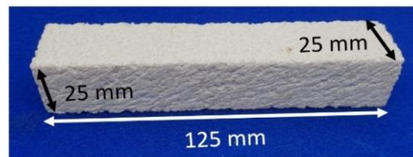
Figure 20: Specimen dimensions for Young's modulus measurements
