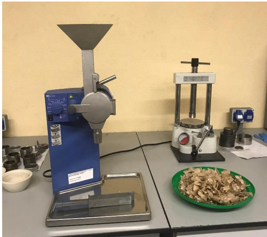
Figure 9: The process of grinding material with the MF 10 basic mill
