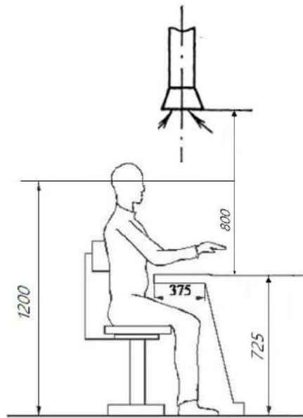
Figure 3. The workplace of the electric and gas welder.
