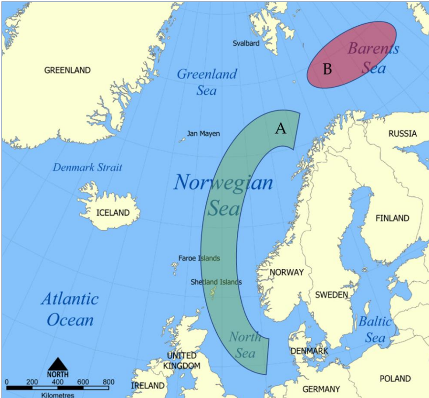
Figure 22: Overview of creeping and non-creeping formations in the North Sea, the Norwegian Sea and the Barents Sea: A – creeping formation area; B – non-creeping formation area (Fredagsvik 2017).
