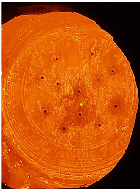
Figure 5.28: BOF bottom stirring elements after relining (12 of 12 available).
