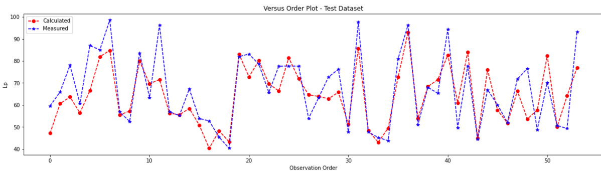
Figure 5.36: Dataset test for the Phosphorus partition ( L_P ) model, calculated versus observed values.
