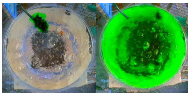
Figure 4.8: Mixing time determination for bottom stirring experiments through the colorimetric method.
