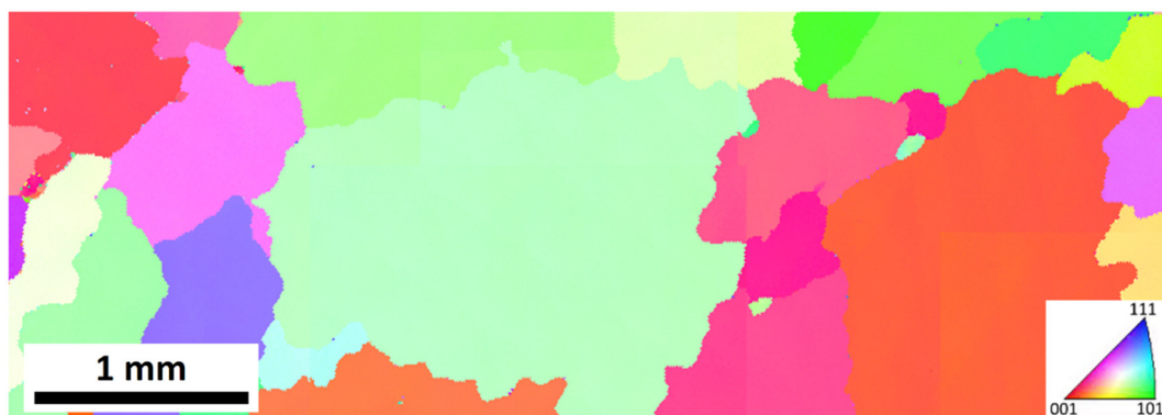
Fig. 5.1: Stitched IPF map of the coarse-grained microstructure on a pure Mo sample.
