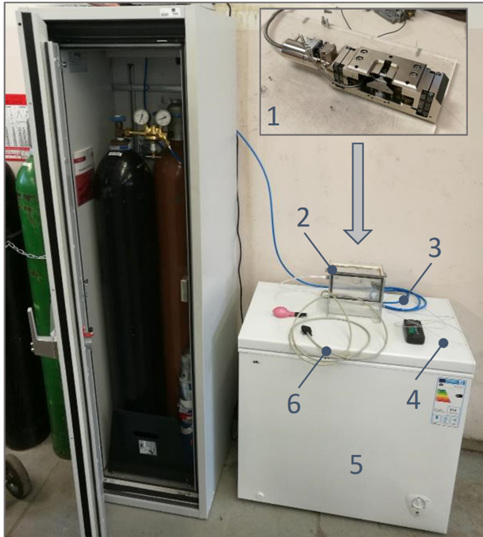
Fig. 3.3: The experimental setup for low-temperature meso-scale bending experiments. The K&W bending module (1) is placed in a desiccator (2), where N_2 gas flow (3) can be introduced. A thermocouple (4) is placed near the sample and the closed desiccator is positioned inside the cooling chamber (5). The motor control and data acquisition (6) as well as temperature measurement (4) is lead out of the cooling chamber and the bending experiment is started after reaching the target temperature.
