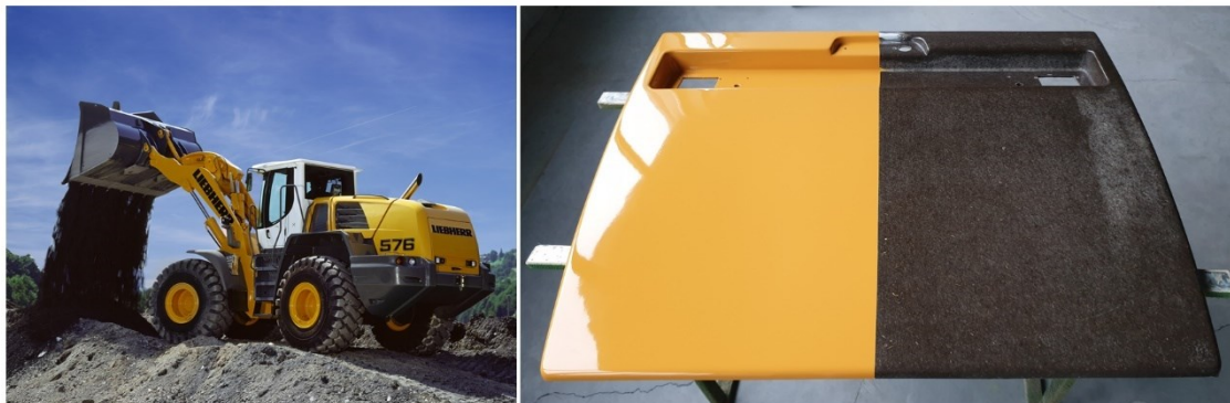
Figure 1: Wheel loader tailgate made of flax fiber reinforced epoxy resin in the frame of the FFG project 'Reliable and Sustainable composite production for Biobased Components' (RSBC)
