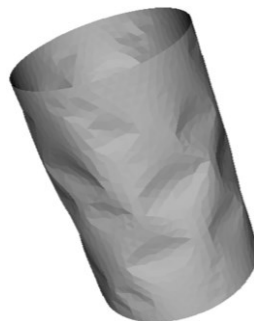
Figure 3-13: FDEM approach applied for the modelling of a cylindrical object (FEM-based/relating shell structure) [182]
