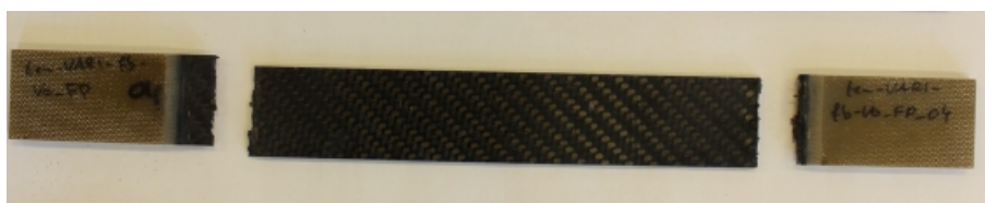
Figure 4.14: Picture of a typically failed fb specimen.
