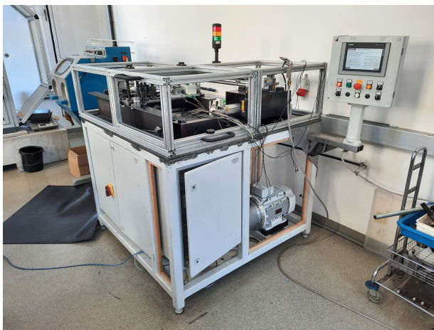
Fig. 2.1: Equal channel angular pressing test bed ©2021 Chair of Metal Forming
