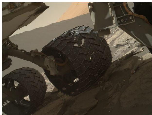
Figure 8.1: Wheel damage on Curiosity [27]
